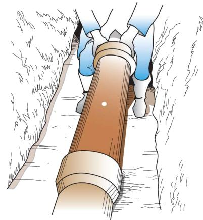
e ) Holes must be dug at each socket (bell hole) to make sure that the pipe barrel is resting firmly on the trench bottom or bedding material so that load is supported by the pipe barrel and not the pipe socket.
